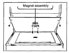
Take out 2 screws holding the magnet assembly and remove the magnet assembly.
